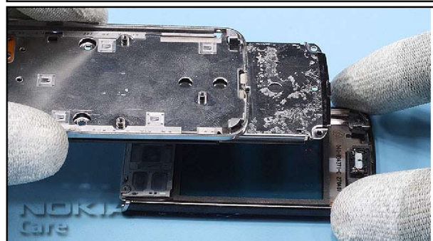
24. Lift up the C-COVER ASSEMBLY.
